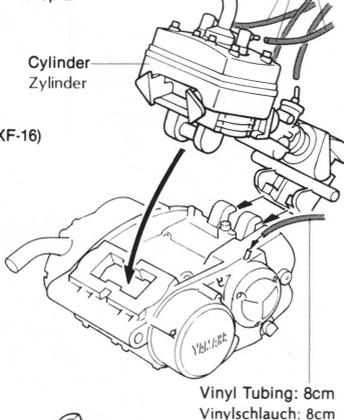
**3** Placing Engine into Frame
