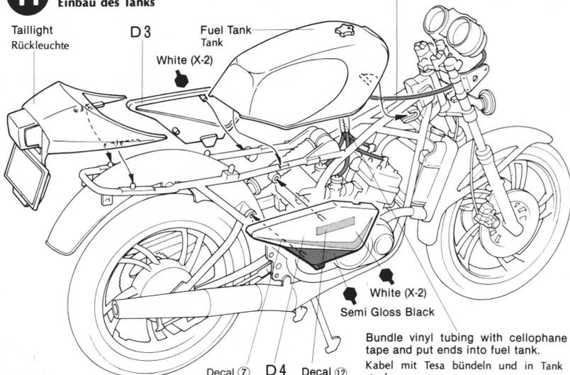
Bundle vinyl tubing with cellophane tape and put ends into fuel tank.
