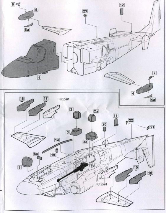
Detail resin set to make the Kamov Ka-50/52. For experienced modellers. Many items have a complex shape and very slim design and require increased care and accuracy in circulation. For best result gluing use cyanoacrylate glue. Not for children.
