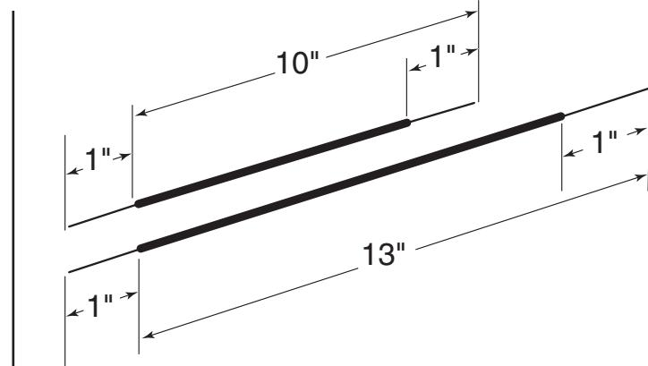
Cut wires to length and strip insulation off as shown.
