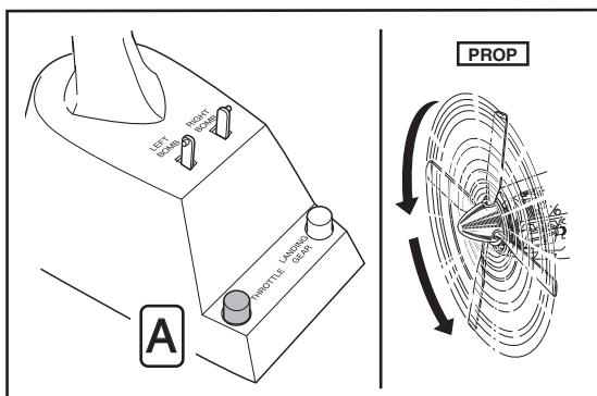
**A.** Press buttons to check operations of landing gear and propeller. Propeller should turn in a counter-clockwise direction when viewed from the rear.
