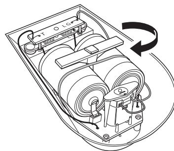
Install two batteries and turn assembly over. Press LANDING GEAR push button to make certain the motor operates freely. "Do Not Press" THROTTLE push button
