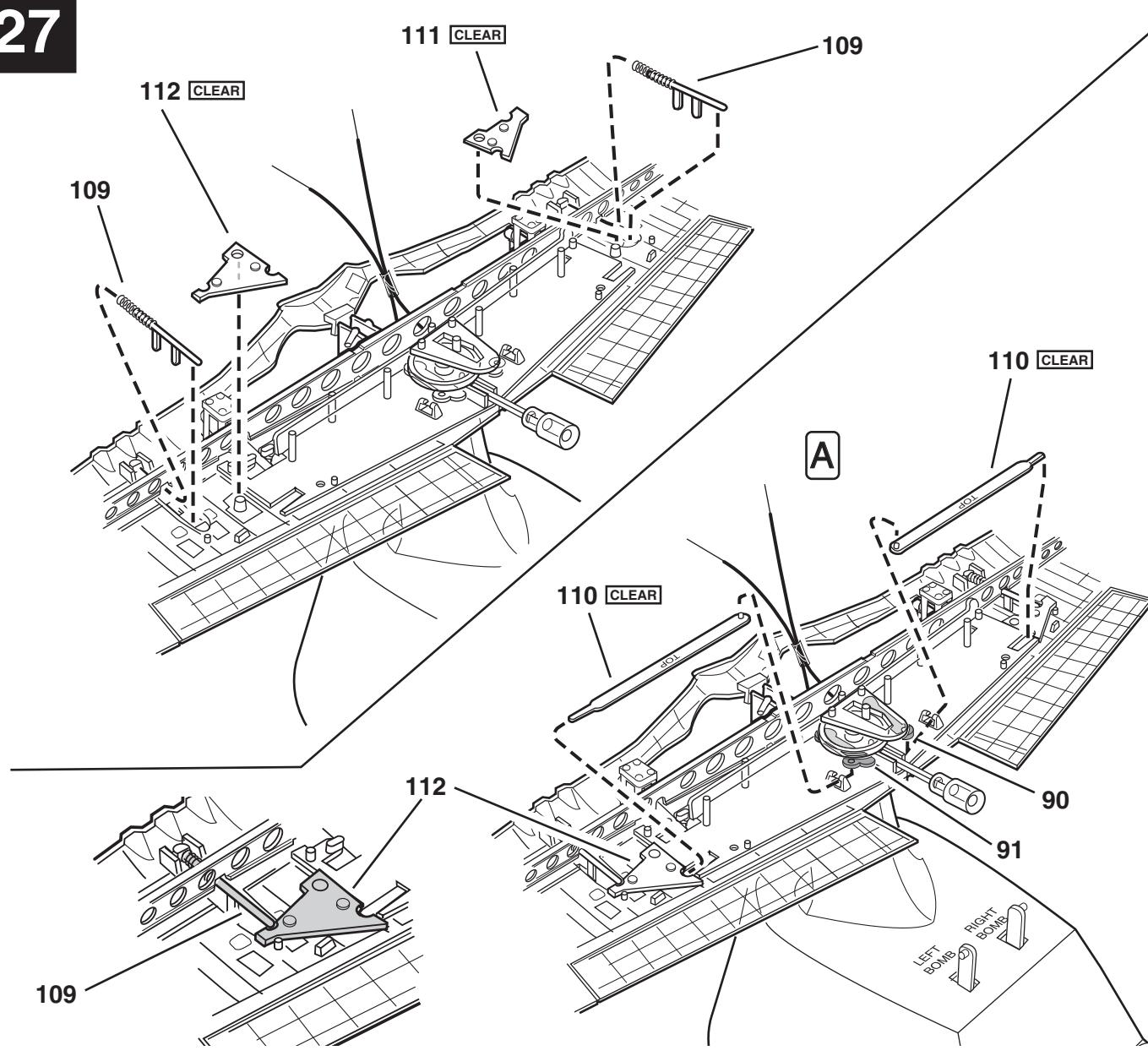
A. Slip part 110 under slot as shown and insert pin into hole in part 90 and 91.
