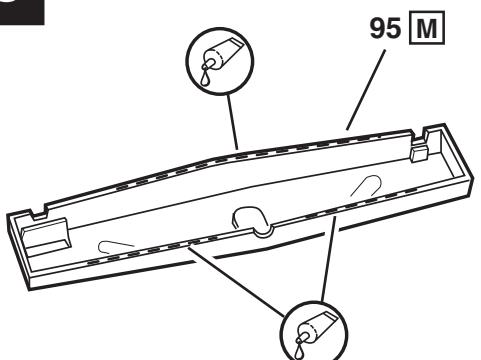
Carefully apply cement along edges indicated by dash lines.
