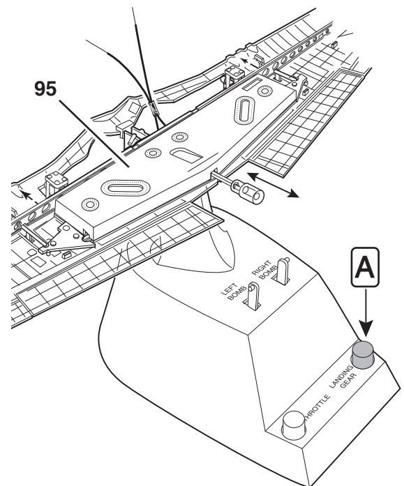
A. Replace part 95 (do not cement) and press landing gear push button to see part 107 moves in and out freely.
