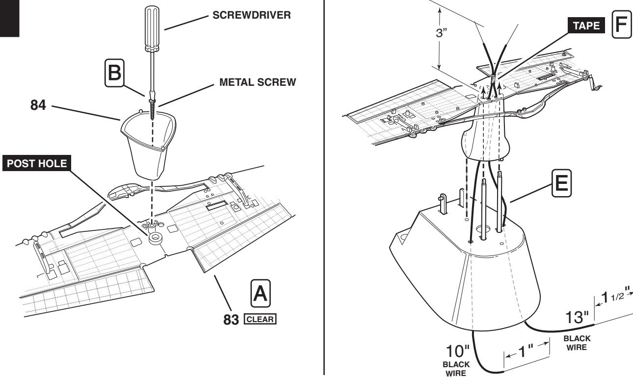
**A.** Carefully turn a screw into post hole in center of part 83 to cut threads into the plastic. Then remove screw.
