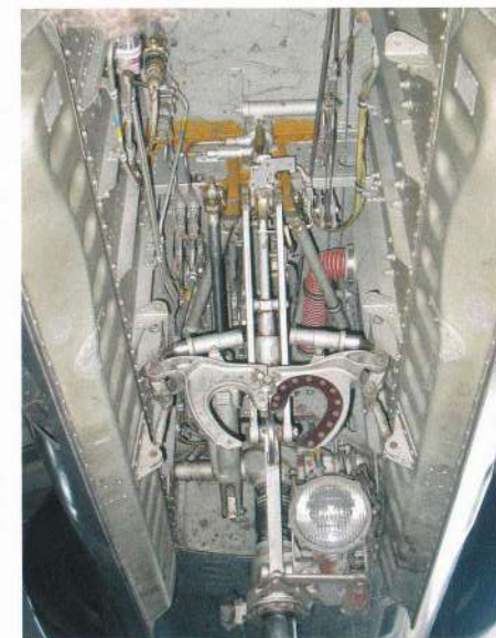
This page: nose landing gear. The swept leading edge of the doors fits into a shallow recess under the fuselage.
