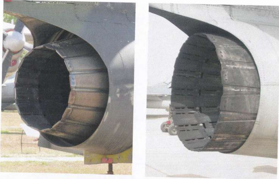
Above: Late type 16-petal afterburner nozzle in closed and open position. Below: The General Electric J79 engine. Right side view.
