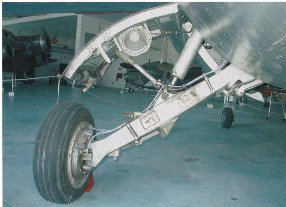
This page: more details of the main landing gear, brake and well. Note the door-mounted landing light.
