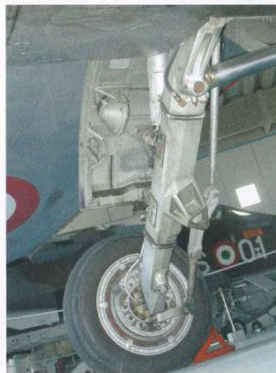
This page: more details of the main landing gear, brake and well. Note the door-mounted landing light.
