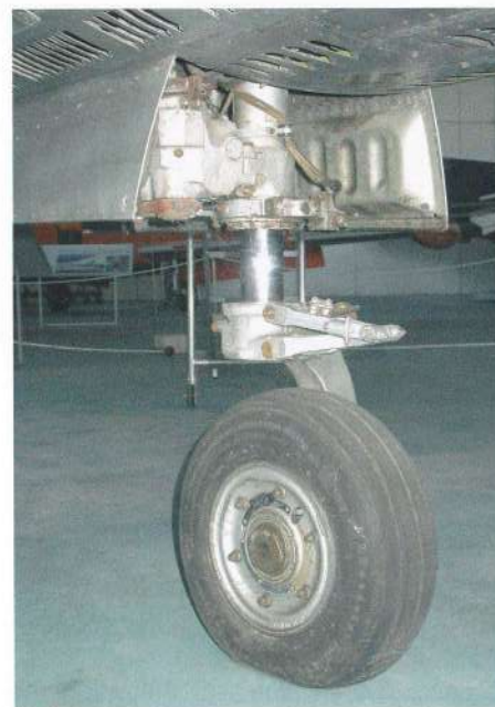
This page: nose landing gear. The swept leading edge of the doors fits into a shallow recess under the fuselage.
