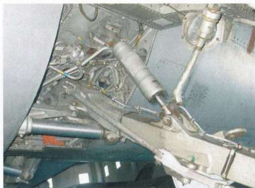
This page: more details of the main landing gear, brake and well. Note the door-mounted landing light.
