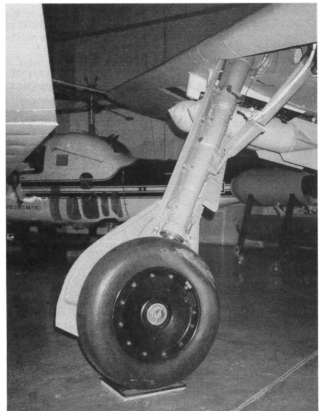
Details of the right main landing gear as used on the Fw 190A can be seen in this view. (Detail & Scale photo by Bert Kinzey)
