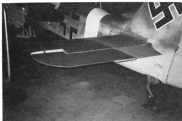
Here is a look at the left horizontal tail. The metal trim tab on the trailing edge of each elevator was painted red. (Detail & Scale photo by Bert Kinzey)
