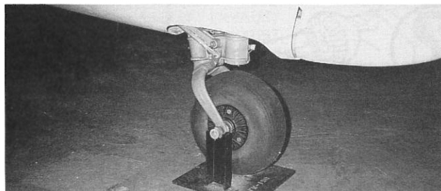
Details of the tail wheel are visible in this photograph. The strut was painted GRAY, RLM 02, and the wheel was dark gray or flat black. (Detail & Scale photo by Bert Kinzey)
