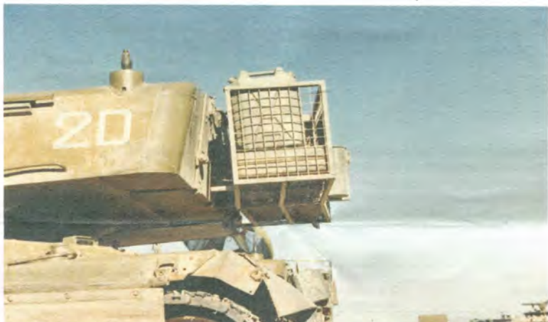
The square turret baskets did not conform to the inward sloping rear turret wall and therefore had stand off legs.
