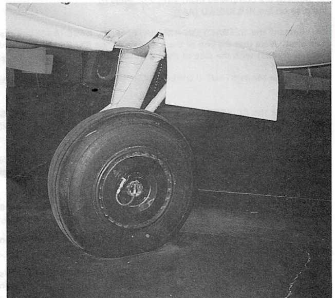
Here is a look at the left main landing gear from the outside. Note that the wheel was painted flat black. (Detail & Scale photo by Bert Kinzey)
