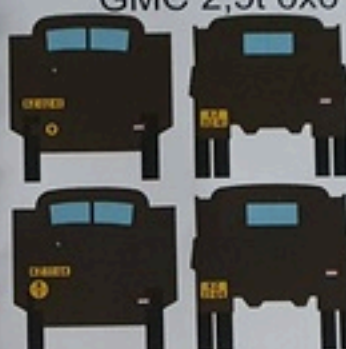
GMC 2,5t 6x6 KZ-02-41, Unknown transport unit. License plates are on a separate plate, attached to the headlight protector, and to the bumper on the rear.
