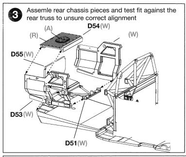
Raise transaxle and slide cage underneath, then glue the cage to the truss.
