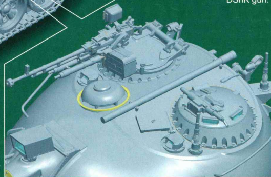
Detailed top turret with 12.7mm DShK gun.
