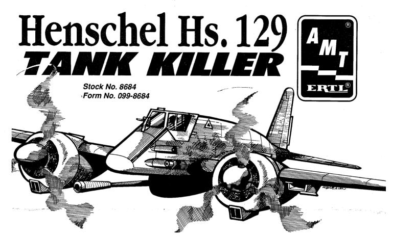
The Henschel Hs. 129 was designed as a single seat, ground attack aircraft. The most unusual thing about the plane is its heavily armoured cockpit. The nose of the 129 bears a striking resemblance to one of today's great ground attack aircraft—the American A-10 Warthog.
