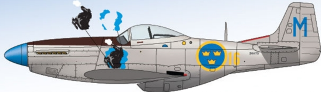
J26, 26075, blue Martin, second squadron F16 Uppsala. Propeller without cuffs (the thick part at the blade rot) Most likely walkway on left wing only. Detached AN/APS-13 antenna on vertical stabilizer (this left a little panel that a/c without the antenna didn't have). The horse badge is separated in two parts to make it possible to use with a/c that did not have the background, blue D for example.
