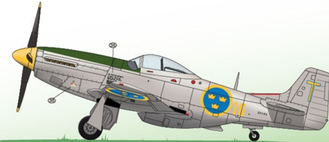
J26, 26049, yellow Tore, third squadron F16. Red fuel caps, low placing of serial number and straight walk-way on left wing only. Most likely green antiglare panel.
