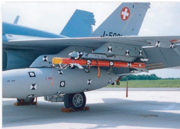
Unique 'low drag pylon' developed to carry AIM-120B AMRAAM on the outboard wing station. This view shows an AIM-9P during an early test. Please note the intensive use of additional photo reference markings.
