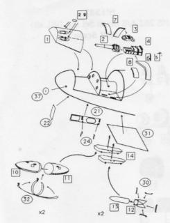
File down front of kit part H14 to receive 1 Add weight to the nose area to avoid Tail-sitting Cut mounting tabs on kit before installing guns Slice end of 2 if 1 s to be used.
