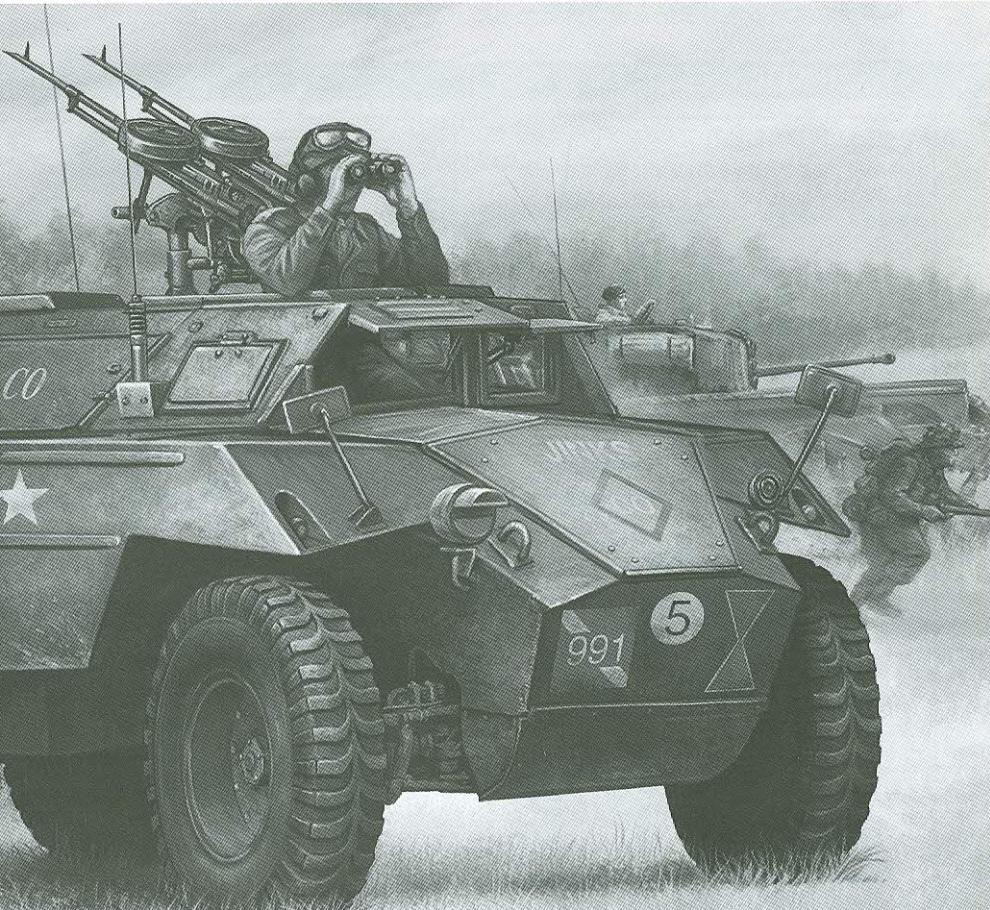
The role of the Daimler Scout Car was expanded 1942-43 to include Scouting, Liaison and Forward Reconnaissance, and so the production of the little vehicle could not keep pace with the increased demand. Humber were asked to build Scout Cars to fill the need, but instead of copying the Daimler, produced their own slightly larger vehicle using many components already in production. The result was the Humber Scout Car MkI, which appeared in early 1943.
