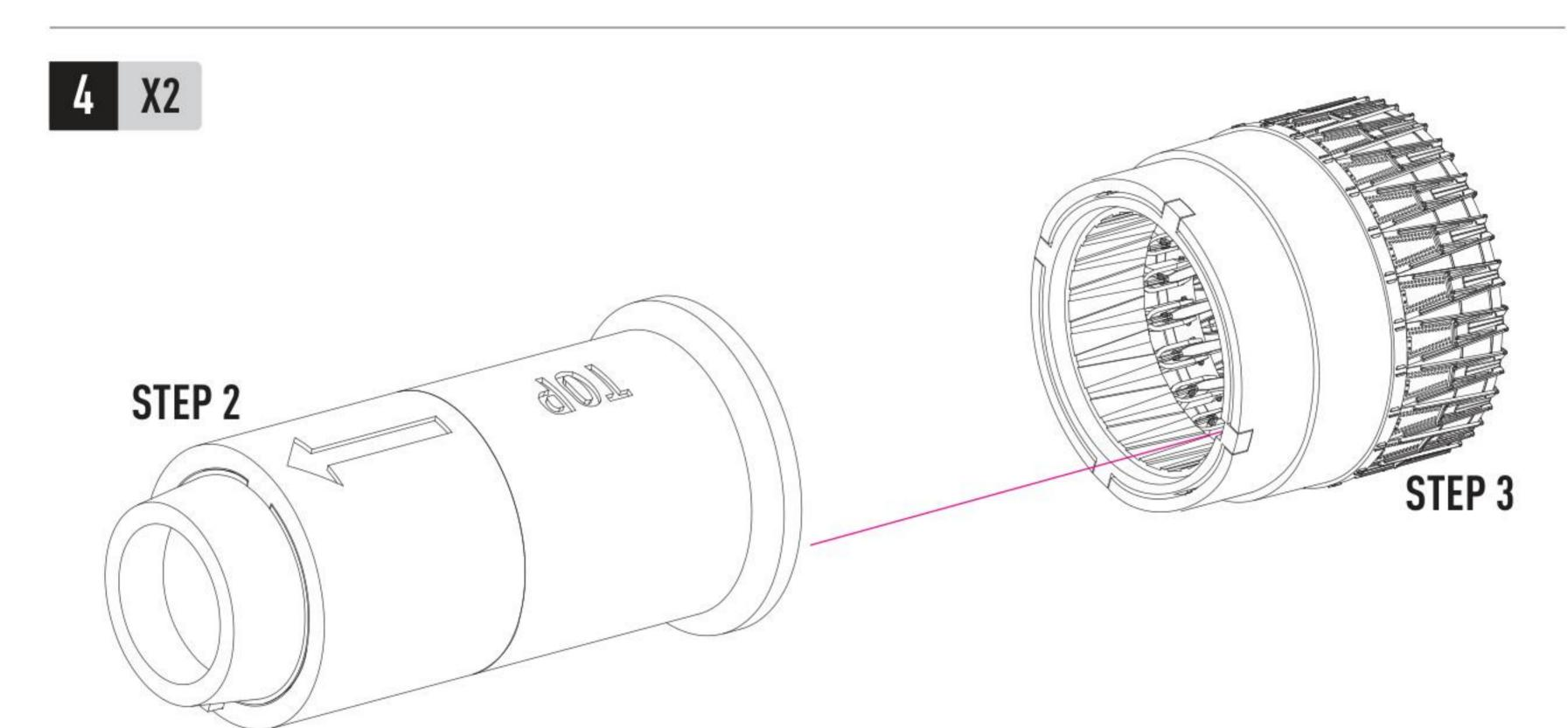
INSTALL THE NOZZLES INTO COMPLETE FUSELAGE PART USING FINEMOLDS PLASTIC KIT PART A30 INSIDE THE FUSELAGE FOR PROPER NOZZLES POSITION
