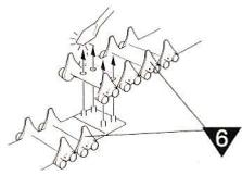
\* Melt pins together with a heated screw driver.
