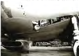
●脚收納庫に取り付けられた着陸灯。 前縁にはガンカメラが見える。 The landing light was installed in the main landing gear well. The gun camera can be seen in the wing leading edge.
