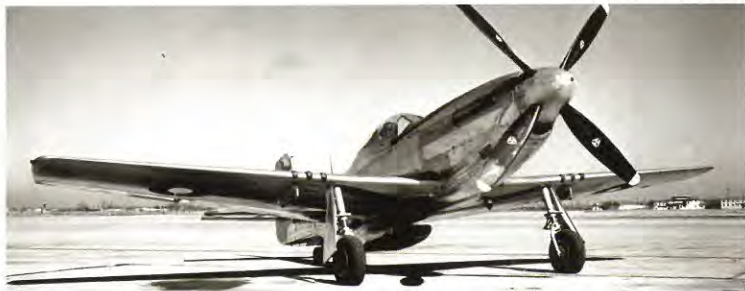
●エアロプロダクツ社製のプロペラを装備したP-51K。 The P-51K was equipped with an Aero products propeller.
