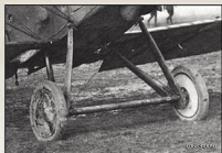
Late wooden undercarriage from rebuild RE.8 H7139. Wooden undercarriage legs were usually left unpainted with black metal brackets. Note the heavily stained starboard wheel cover, possibly from oil spilled when filling the tank immediately above.
