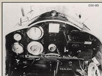
Instrument board showing one style of arranging the instruments. Note the small lamps for illuminating the instruments when night flying, RAF Mk.II compass, Very flare pistol holster and tailplane trim wheel on the right. Uncommonly the mounting brackets for the Aldis sight are positioned on the left of the windscreen.
