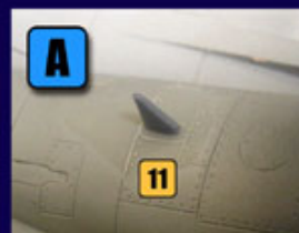
(A) Fuselage Antenna
