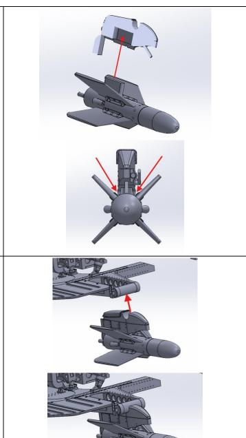
Fix the SS11 launch rail to the front spar of the weapons platform.
