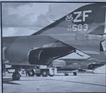
DETAILS OF THE AFTERBURNER NOZZLES ARE SHOWN HERE. THIS PHOTO ALSO SHOWS THE VARIOUS SHADES OF METAL ON THE AFT FUSELAGE OF THE PHANTOM (DETAIL & SCALE PHOTO BY BERT KINZEY)
