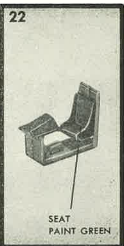
Paint seat green and cement it to panel and floor unit as shown.
