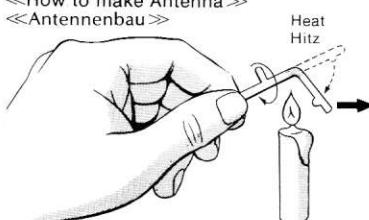
\*Heat a length of sprue and when melted a little, stop heating to stretch it. Hold for about 15 seconds to cool.
