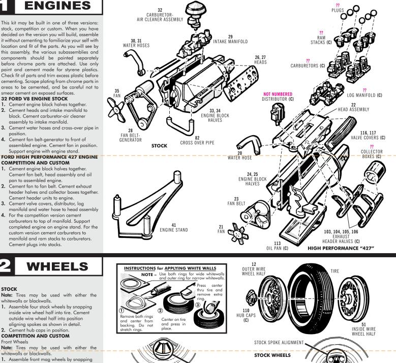
whitewalls or blackwalls. 1. Assemble front mag wheels by snapping inside mag wheel half into tire. Cement outside mag wheel half into position aligning spokes as shown in detail. Rear Wheels
