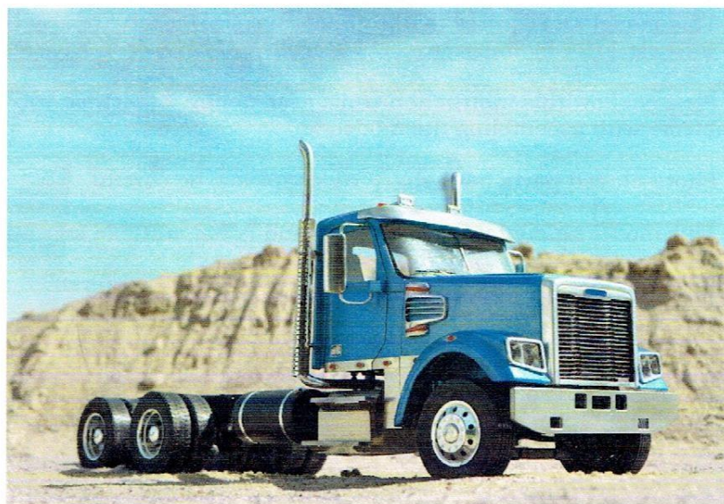
Modern American Conventional truck. (day cab, set forward axle version)
