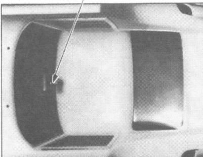
Set the car mirror D15 after the window glass has been cemented to the body.
