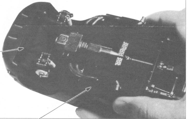
Set the chassis to body while opening both sides of the body
