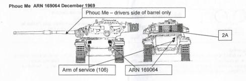
2A was situated on a piece of metal on the turret stowage basket. Place the decal on a piece of olive drab painted 10 thou plastic and when dry cut to size at attach.
