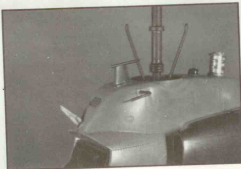
Antennas and Pitot tube are installed
