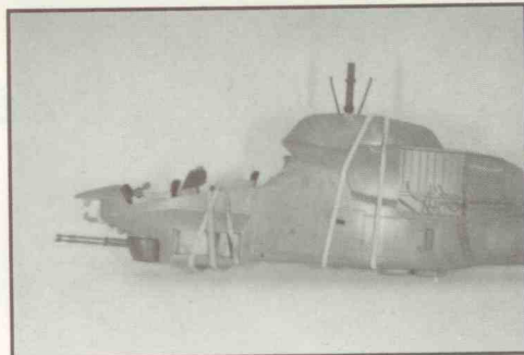
The assembly can be held together until dry as shown above using rubber bands
