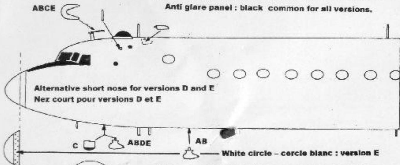
Place a 90 grs lead balast behind the cockpit
