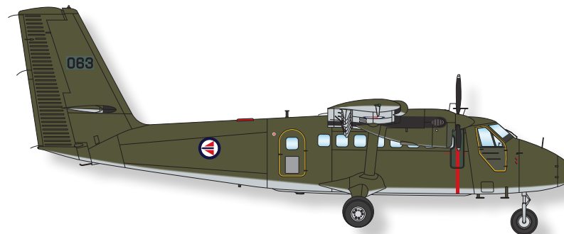
de Havilland Canada DHC-6-100 Twin Otter, 67-063/063. 719 Sqn., Bodø 1988. Window for camera installed in right side cabin door and rear fuselage floor.
