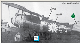
Paul Bäumer's Jasta 5 Albatros D.V photographed at Boistrancourt. Note the 160hp Daimler-Mercedes D.III engine, the fairing over the empty belt chute and Bäumer's edelweiss marking. The different tones of the dark rear of the fuselage are thought to simply be the difference between gloss and matt paints applied at different times.
