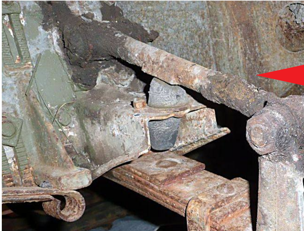
Support arms A35 are longer in the kit, their length needed depends on work accuracy so you might need to make them shorter by cutting the end
