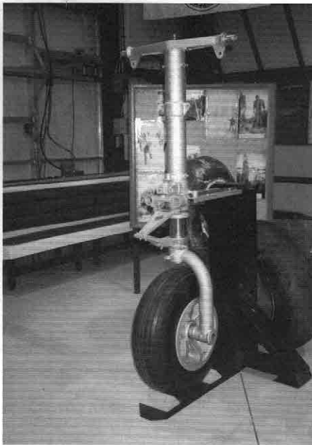
Details of the nose gear strut, wheel, and tire are revealed in this photograph. The strut is painted aluminum, and the oleo portion is bright silver. (Detail & Scale photo by Bert Kinzey)
