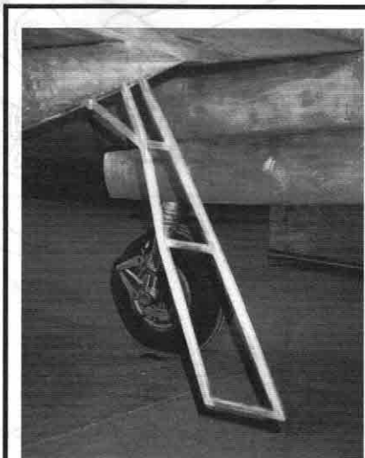
A retractable boarding ladder was located at the aft end of the center fuselage section. This photo shows the correct angle for the ladder when it was in the fully extended position. (Detail & Scale photo by Bert Kinzey)
