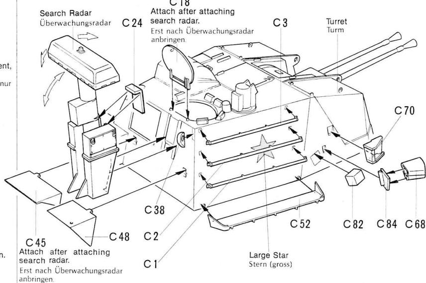
**10** Attaching Tracking Radar
