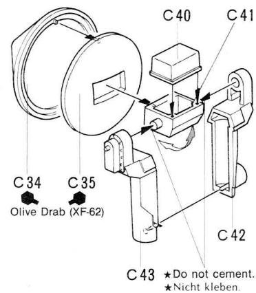
**8** Attaching Gun Barrel
