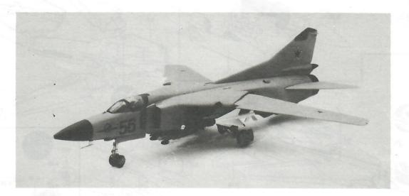
With the successful development of the American F-111 swing-wing fighter, Russian designers utilised the technology to produce their first aircraft of this type. The MiG 23 bears a superficial resemblence to the American design, but is powered by a single jet engine, instead of two, and carries but one crewman.
