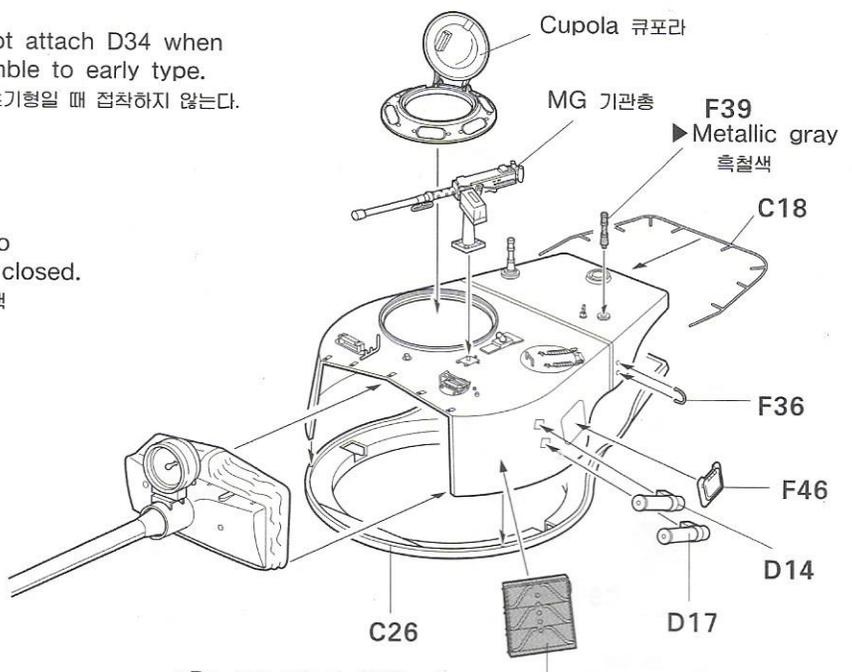
\* Do not attach D34 when assemble to early type.
