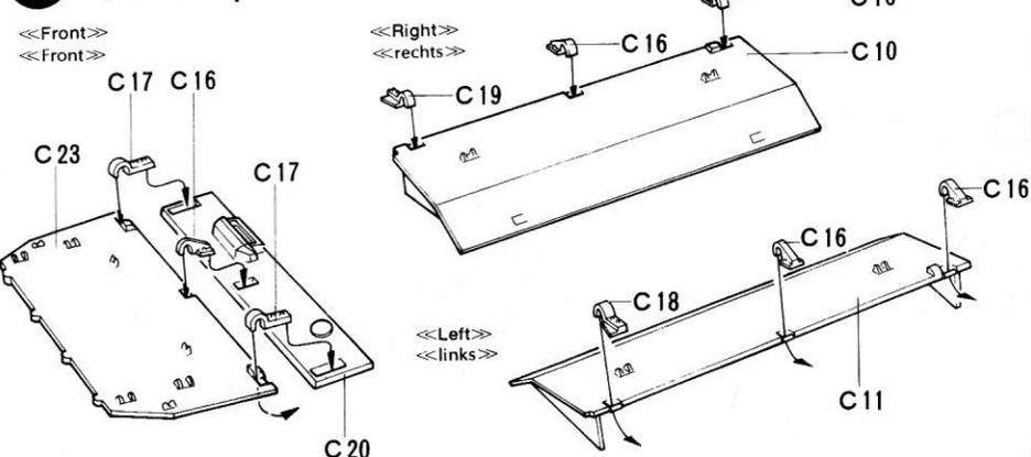
**9** <<Construction of Armour Plates>>
