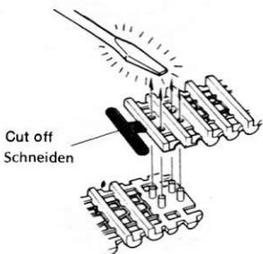
Immediately after that, press pin heads. Sofort Zapfen gerade pressen
