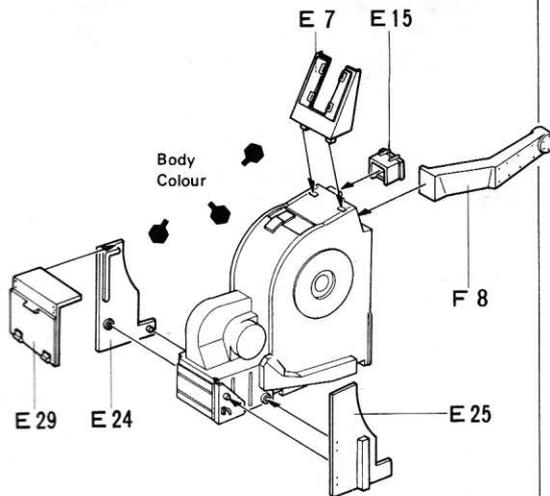
**13** <<Construction of Machine Gun Bases>>
