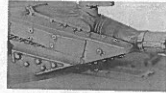
Rivet Detail on Turret
