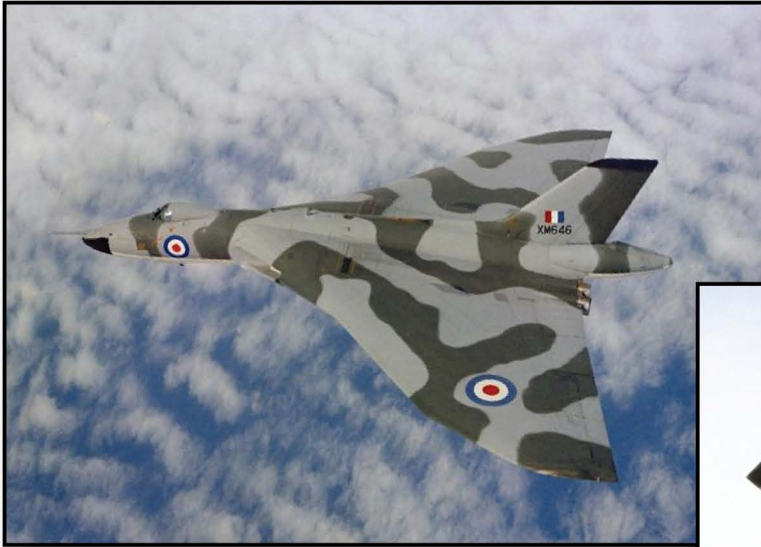
XM646 shows off the typical appearance of a Vulcan during the centralized servicing period from 1964 through around 1972. Her camouflage follows the standard pattern, but appears to have feathered edges between the Dark Green and the Sea Grey Medium, unlike most Vulcans of the time. Radomes are semi-gloss black, and the Type D roundel only appears above the left wing. This view also shows the shorter, larger diameter Olympus 301 series exhaust pipes. Compare to the photo at right.
