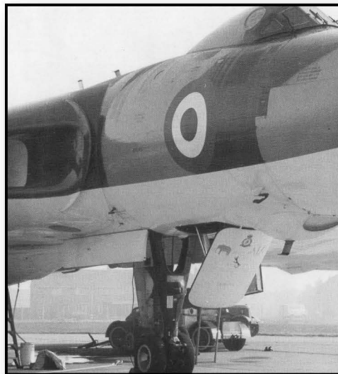
A Vulcan from the Scampton wing during the centralized servicing period. On the crew entry door are the Scampton station crest at the top, surrounded by the badges of 27, 83, and 617 Squadrons. Note the lack of an ejection warning triangle.
