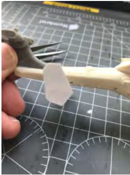
New tailplane fins fitted. This is a very quick modification and makes a big difference.
