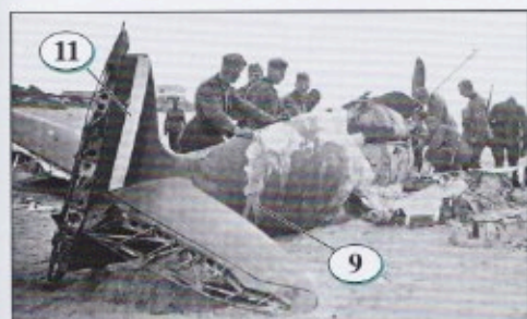
Another view of the wreckage of N3180 showing the rear fuselage and tailplane, which has had its fabric ripped off by victorious souvenir hunters. The style and size of the rudder stripes applied by 54 Squadron at this time is quite apparent.
