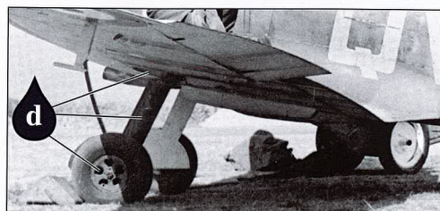
Port side view of the undercarriage from mid-production 19 Squadron Spitfire Mk.Ia P9386 QV-K photographed in September 1940 as seen on page 28. The undersides have been overpainted with a mix of "Sky Type S" and, as is typical of unit repainted undersides, the undercarriage struts, wheel wells, wheel hubs and insides of the doors retain their original factory applied colours of Night and white.
