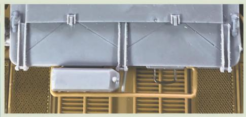
Add two U-shaped supports 4 mm wide x 3 mm deep at the bottom of the rear turret bin.
