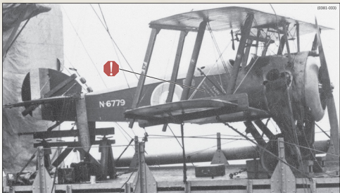
150hp Bentley BR.1 powered Sopwith 2E1 Camel N6779 is from the same Beardmore production order as B and is shown here aboard HMS Calliope in May 1918. Note the illegible "Pilots..." notes written on the side of the fuselage, perhaps not unique to HMS Calliope. See also page 22.
