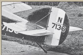
Fin and rudder detail from Sopwith 2.F1 Camel N7136 as seen on page 18. Note the tie down rings under the fuselage.
