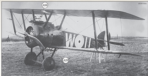
130hp Clerget powered Sopwith F.1 Camel B6355 "W" of "C" Flight 3 Sqn RFC wears the unit marking of 2 vertical bars behind the fuselage cockade. B6355 was captured on 6 November 1917 and its pilot, AG Gribb, was made POW. Note the bomb carrier under the fuselage and position of the Rotherham petrol pump on the front starboard cabane strut.
