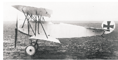
Fokker V 11 prototype, also designated V 11/I in its original form in Autumn 1917. (Albatros/PL Gray Collection-used with permission)
