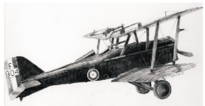
British SE 5a, powered by Wolsley W.4A Viper 200 hp engine, max. speed 222 km/h
