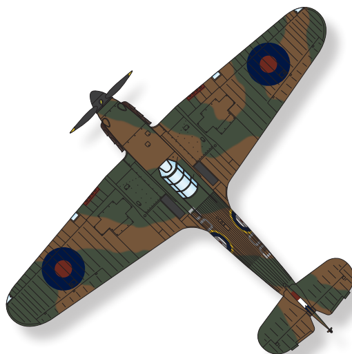
Hawker Hurricane fabric wing with A scheme camouflage pattern. Dark Green and Dark Earth. Dull coloured wing roundels.
