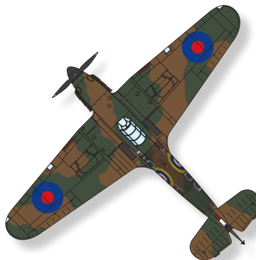
Hawker Hurricane metal wing with B scheme camouflage pattern. Dark Green and Dark Earth. Bright coloured wing roundels.
