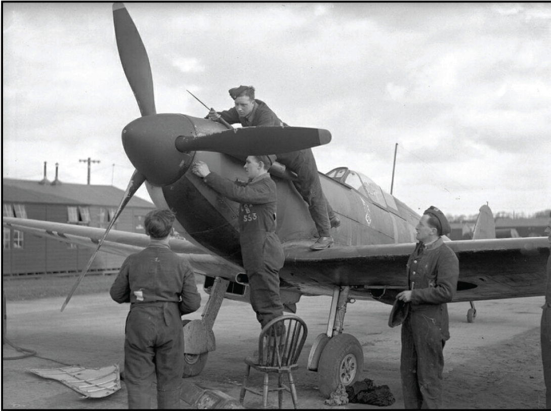
A quartet of 'erks' giving K9955 some loving care at Drem. Note the color of the landing gear legs, wheel hubs, the inner surfaces of the gear doors, and the sliver of the left main gear bay that is visible - all appear to be painted silver. Also note the antenna mast, the external armored windscreen, and the sheet metal L shaped blinkers on the cowling. The aircraft was less than a year old when this photo was taken, yet she appears somewhat scruffy. The Scottish rains undoubtedly made for muddy conditions at Drem, accounting for the splattered appearance of the gear door.
