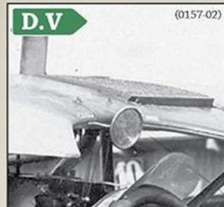
Daimler-Mercedes radiator detail from Albert Tybelski's Royal Prussian Jasta 19 Albatros D.V 2104/17. Note the mirror (E39).
