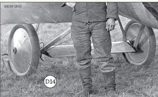
< Undercarriage detail from Albert Dietlin's Royal Prussian Jasta 41 late production Albatros D.V 4612/17 showing the common D.V & Johannisthal built D.Va style of tyre valve access & wheel cover (D14).
